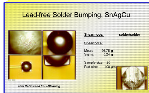
Figure 9: Leadfree Solder Bumping, SnAgCu
