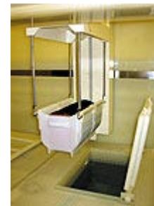
Figure 1. Fifty 200mm wafers are shown undergoing parallel batch processing.
