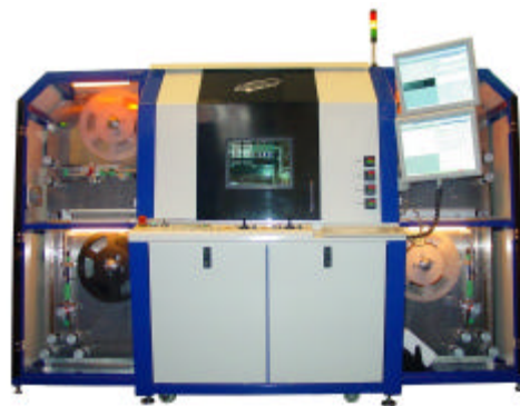
Figure 4: shows a production version of the LAPLACE system with integrated reel – to – reel tool for 35 mm tape and laser class 1 enclosures.
