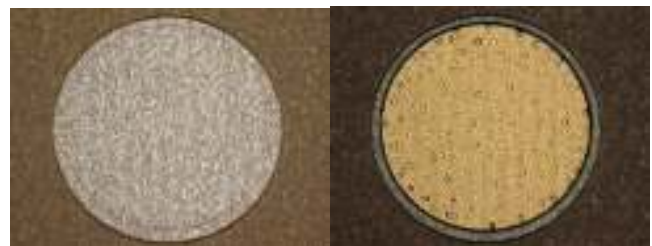
Figure 3. Top View of an Aluminum Bond Pad (left), and Electroless Nickel/Gold Plated Bond Pad (right).
