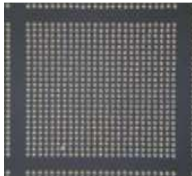
Figure 6. SEM Image of 100µm Flip Chip Bumps.
