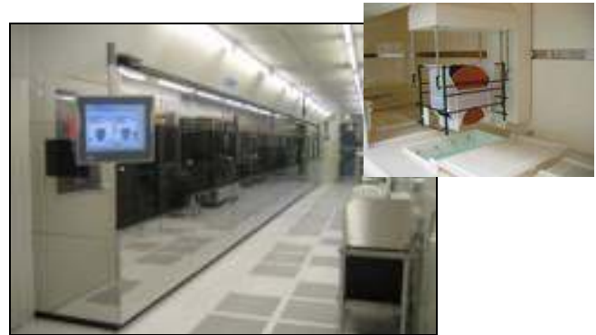
Figure 2. Electroless Nickel Plating Line (Pac Tech PacLine 300 A50).
