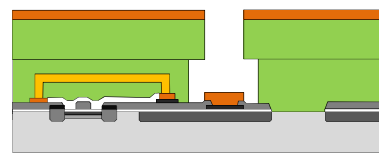
Step 2. Sputter deposit 500 Å of Ti followed by 6000 Å of Cu.
