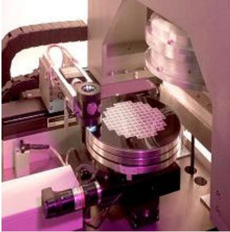
Figure 2. Close-up view of the SBT tool (PacTech Ultra-SB2).
