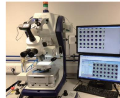
Figure 4: Test setup for BST testing. The wafer samples were secured using a vacuum wafer chuck.
